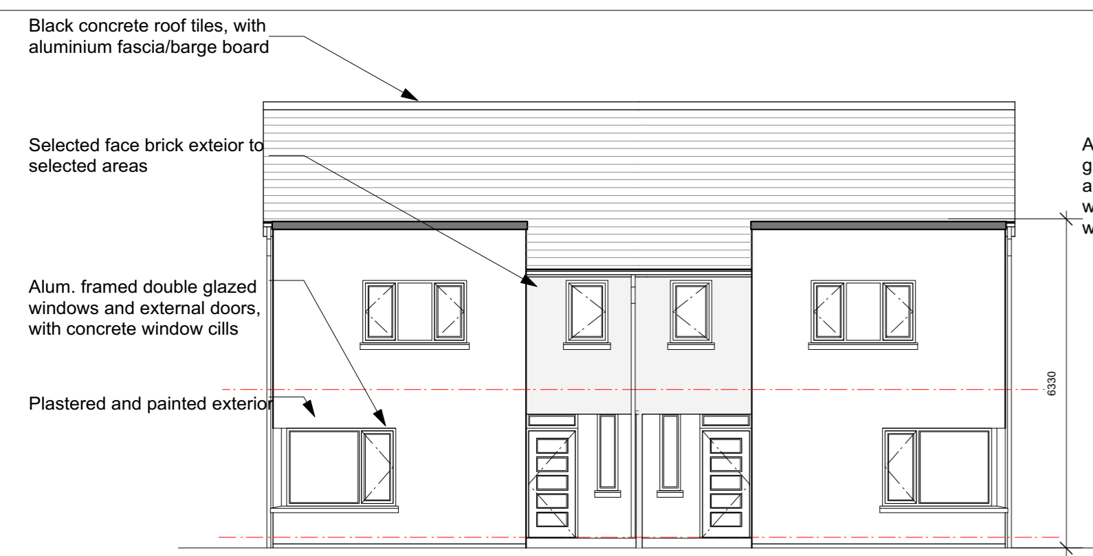
1 Semi-Detached Proposed Front Elevation Scale 1:100
